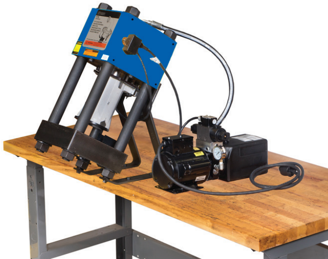
Figure 8 Typical ET4001 equipment set-up on shop/work table
