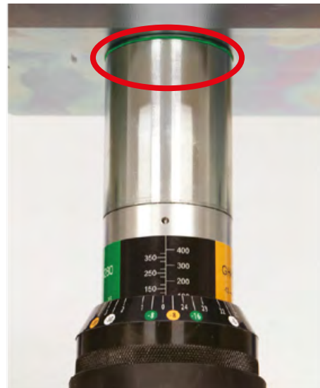
Figure 6 Crimp cycle is complete when cylinder travel stops and the green indicator ring on the piston shows beneath the top plate. After completion, visually inspect the crimp and verify the correct crimp diameter and length.
