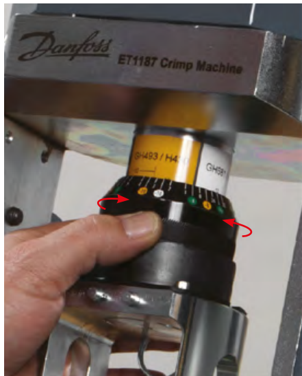
Figure 4 Rotate crimp adjustment ring until desired dash size is lined up with corresponding dash size on product selection collar.
