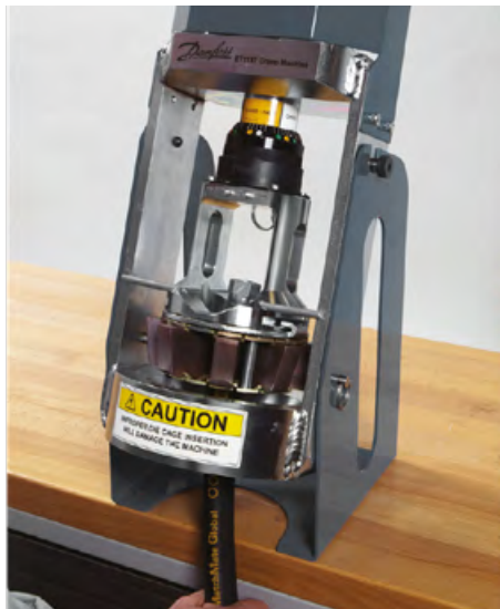
Figure 5 Insert the hose assembly up through the bottom of the base ring and die cage. Begin crimping by actuating the pump.
